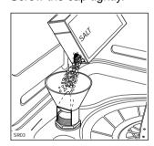
When this has been done, all that is required is to periodically add salt to the container. You are reminded of this by the Salt refill light **«SALT»** on the control panel which will illuminate when the salt has finished.
